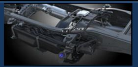
To meet stringent Canadian emissions requirements, Ram Chassis Cabs with the Cummins Turbo Diesel engine are equipped with a Diesel Exhaust Fluid (DEF) injection system and a Selective Catalytic Reduction (SCR) catalyst. When needed, the DEF is injected into the exhaust to reduce NOx (Nitrous Oxide) emissions coming out of the tail pipe. Low emissions allow the engine to idle practically indefinitely on the jobsite, giving you use of HVAC and electrical features
